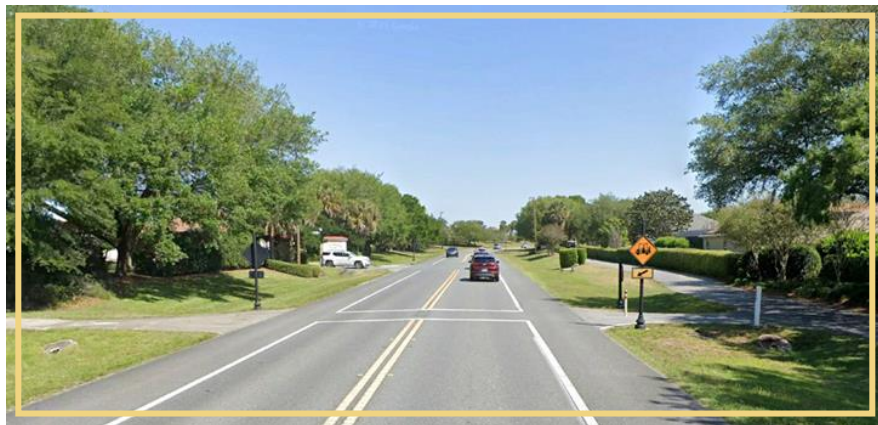
Photograph 5 - Marked golf cart crossing of Morse Boulevard
