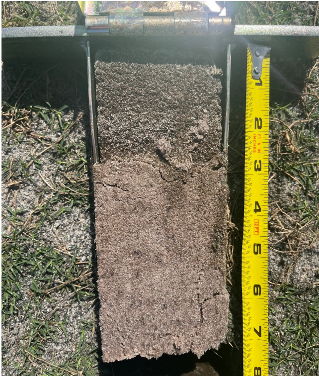
Figure 3: Profile from Bonita Pass showing a 3" thick organic matter layer.
