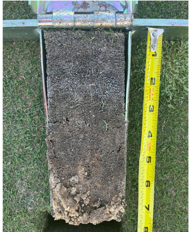
Figure 2: Profile of an older putting green with over 6" of organic matter layer on Pimlico.
